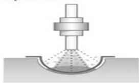
The hole is filled with a mixture of aggregate and asphalt
