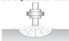
The Jetpatcher blows any loose debris out of the pothole
